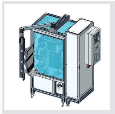
The spindles are arranged vertically to enable optimum clamping. The larger cross-sections of the spindles require an opposite arrangement. This means that very small centre distances can also be realised and the measuring device is thus also suitable for measuring internal gears. The drive takes place at the master gear, the workpiece is braked.
